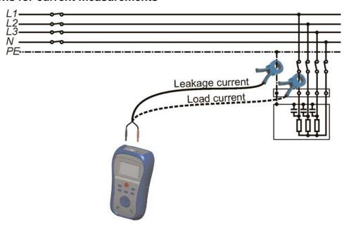
Figure 5.12: Leakage and load current measurements
