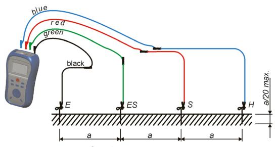
Figure 5.9: Specific earth resistance measurement
