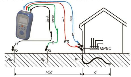
Figure 5.2: Resistance to earth, 4-wire measurement of main installation earthing
