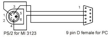
Figure 6.12: Interface connection for data transfer over PC COM port
