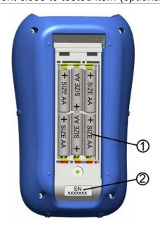
Figure 3.4: Battery compartment
