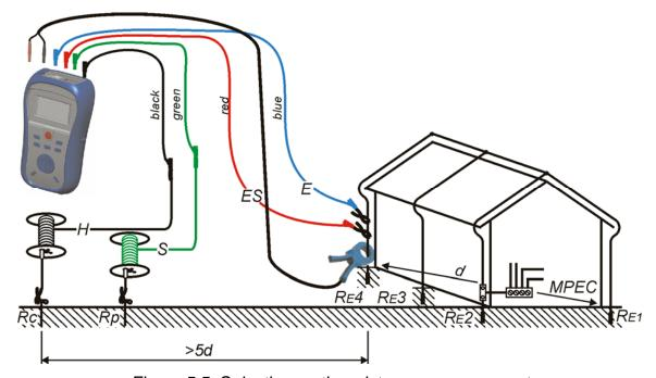
Figure 5.5: Selective earth resistance measurement
