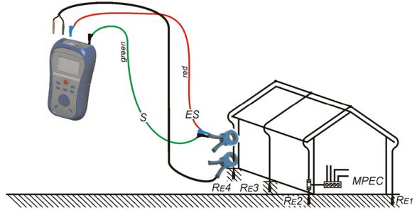
Figure 5.7: Contactless earthing resistance measurement
